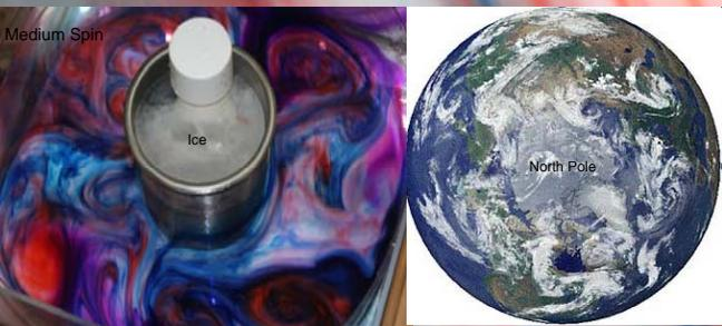
The Hadley cell near the equator is characterized by warm air rising and flowing away from the equator and cool air sinking at mid-latitudes and flowing toward the equator. In our experiment, cool water sinks to the bottom of the tank flows out, while warmer water on top of the tank flows toward the ice (away from the equator). The Coriolis force from the rotation then causes a shear in this flow and water at the bottom and top of the tank flows in opposite directions around the ice.
